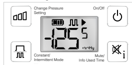
Pomp in intermitterende modus (aan)
