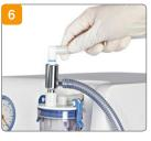
Plug the supplied tubing into the 3-way adapter.
